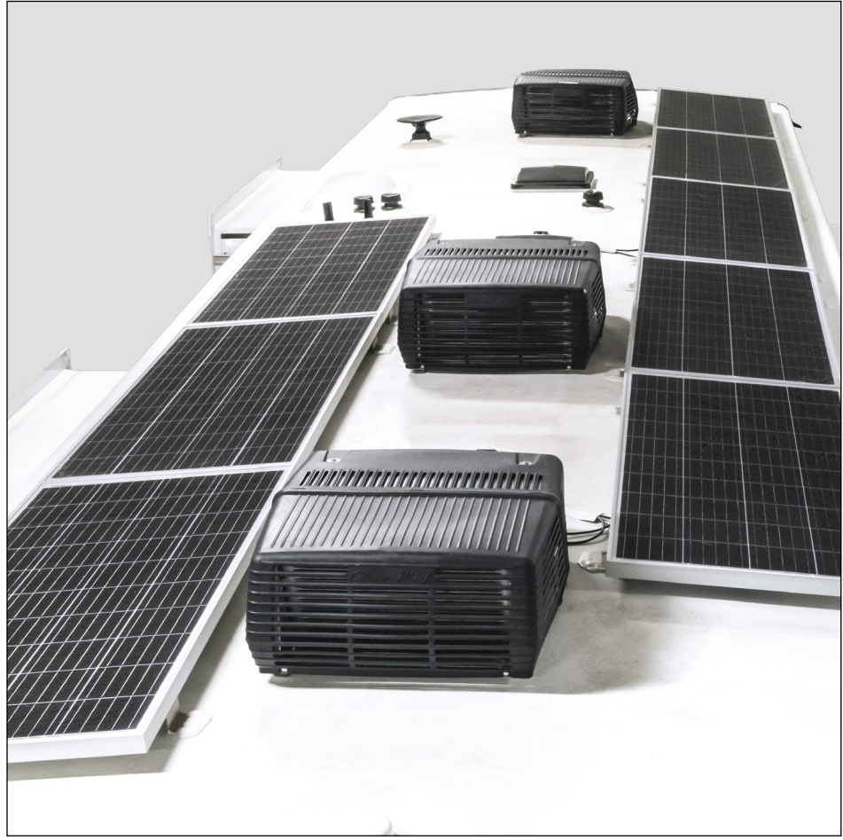
(10) 200W solar panels = 2,000 Watts of solar power
