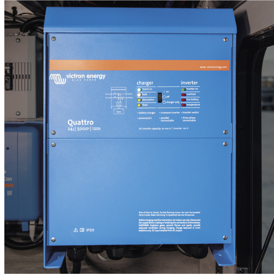
5,000 Watt Victron Inverter/Charger 48V - powers everything in your fifth wheel + (1) 15,000 BTU A/C with Soft Start
