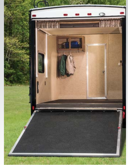
(Right) Ramp transitions include a beaver tail for easy loading.
